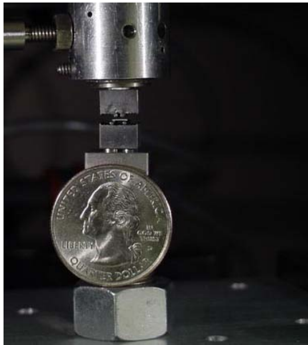
Fig 4.2. Micro-bend configuration actuated by a nanoindenter. The four pins of the 4-point bend can be seen end-on.
