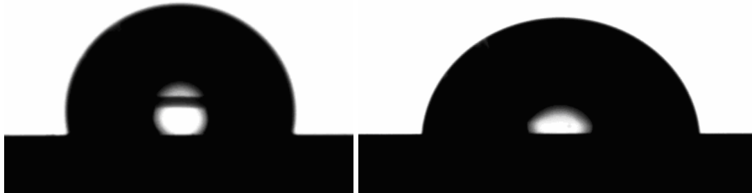
(b) Advancing contact angle under visible light (c) Advancing contact angle under UV light
