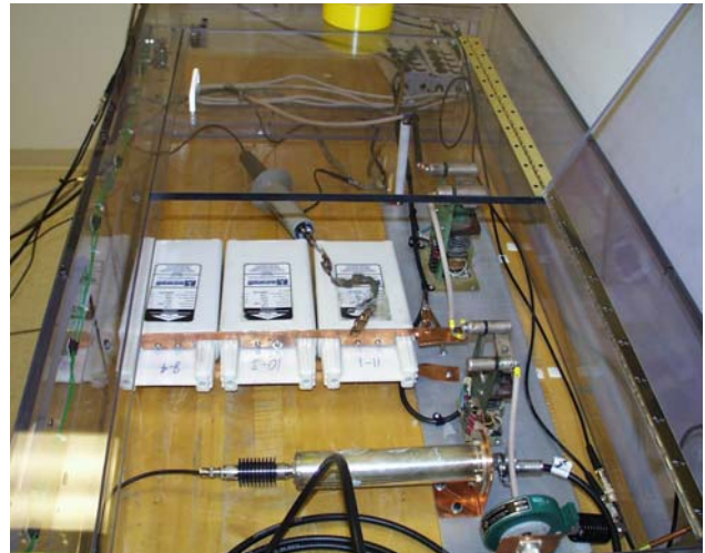
Figure 12. Large energy deposition experimental layout. Energy storage capacitors are white objects in center, current monitors are shown below.
