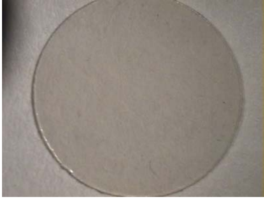
Figure 55. Microscopic photograph of a mylar sample before a high energy discharge.
