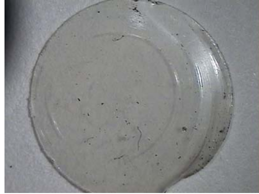
Figure 52. Microscopic photograph of a mylar sample after a low energy breakdown.
