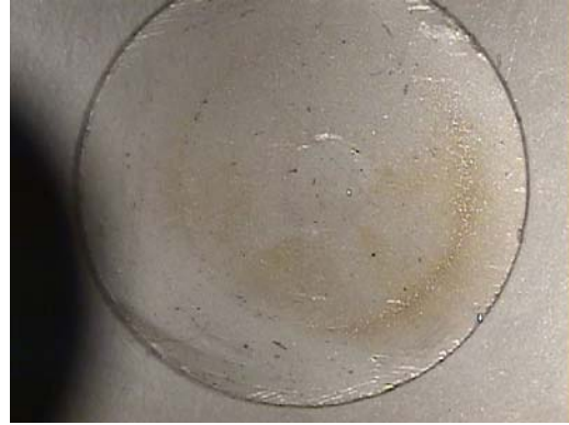
Figure 56. Microscopic photograph of a mylar sample after a high energy discharge.
