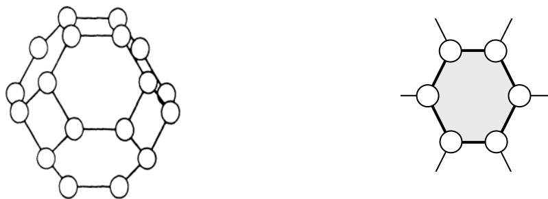
Figure 10: (left) A three-dimensional, idealized grain-pore geometry used in the Coble[23] phenomenological model for final-stage sintering showing spherical pores at each apex of a tetrakaidecahedron-shaped grain, and (right) its common two-dimensional representation.[31].
