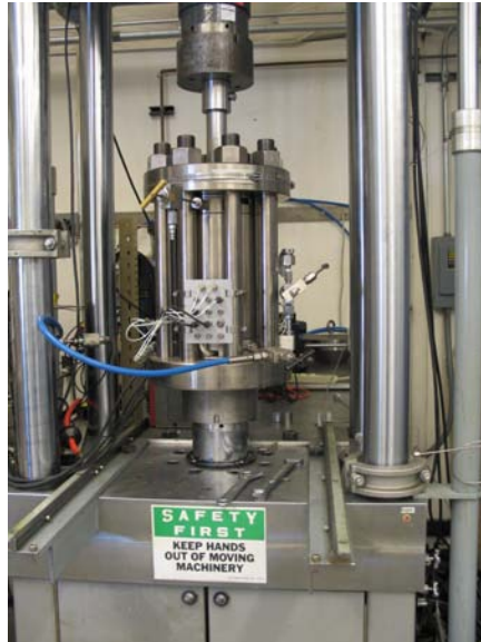
Figure 15. Load frame with pressure vessel in position ready for testing. Axial ( \sigma_{11} ) stress was applied by the piston that passes vertically through the vessel closure. Lateral stress ( \sigma_{33} ) or confining pressure s applied to the jacketed sample by fluid (Isopar) in the pressure vessel.
