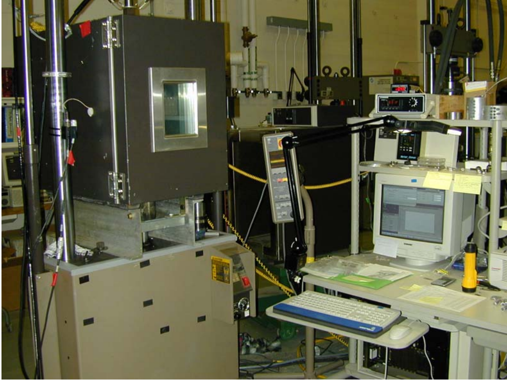
Figure 10. MTS 880 load frame and control system used for tensile experiments.
