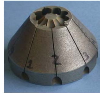
Figure 5. Tensile specimen cylinder removal plan and post-EDM photograph for HERF reservoir forging C.
