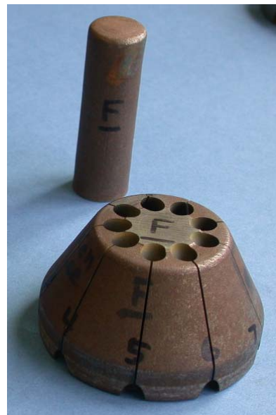
Figure 8. Tensile specimen cylinder removal plan and post-EDM photograph for HERF reservoir forging F.
