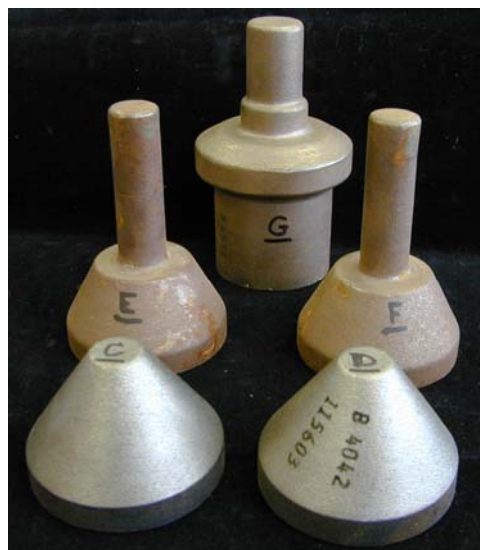
Figure 4. 304L stainless steel HERF reservoir forgings C, D, E, F, and G.
