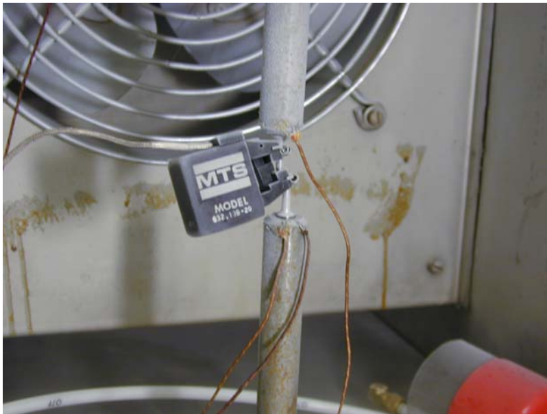
Figure 11. Failed tensile specimen tested at -40^{\circ}\text{F} .
