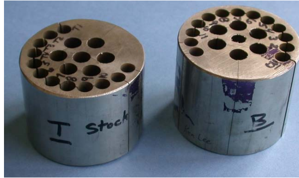
Figure 2. 304L stainless steel bar stock after specimen cylinder blank removal.
