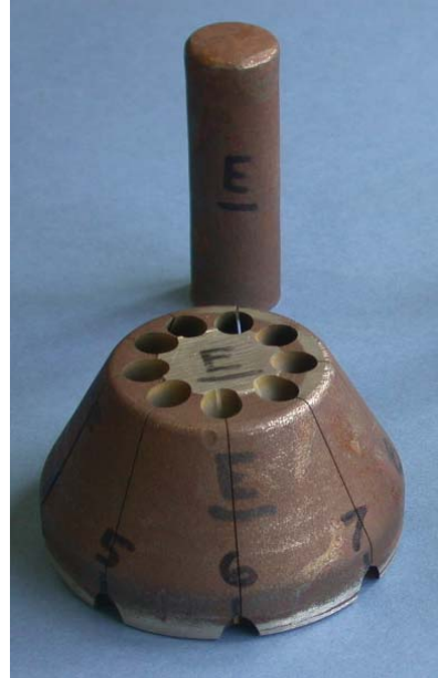
Figure 7. Tensile specimen cylinder removal plan and post-EDM photograph for HERF reservoir forging E.
