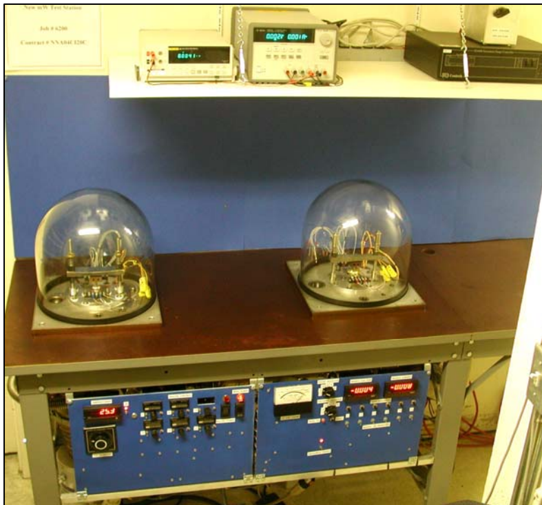
Figure 26. The new test stations run at a pressure of \sim 1 \mu\text{torr} and the module cold side temperature can be controlled down to -10^\circ\text{C} on two stations and -160^\circ\text{C} on the cryogenic station.
