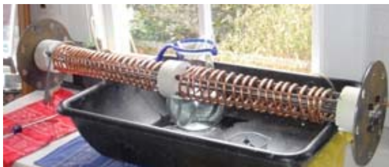
Photo No. 19. Methanol Vaporization System Heat Coil During Fabrication
