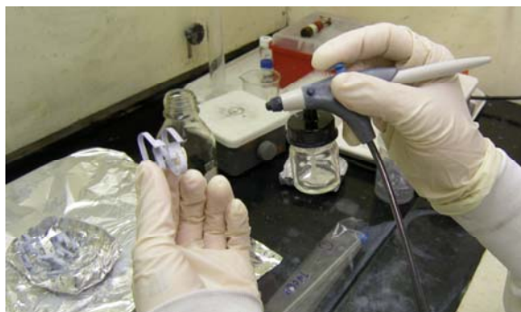
Photo 27. Spray gun used to coat the silica-titania composite on the stainless steel substrate
