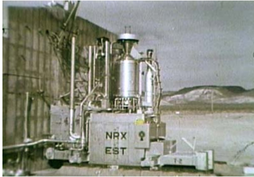
Figure 2. Nuclear Rocket Testing (Nerva Reactor) at Test Cell A Resulting in Activation of the Shield Wall.
