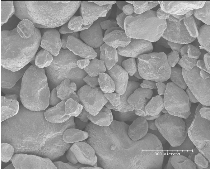
Figure 3.6 (Top) A low magnification back scattered electron micrograph of an indurated region of a MPS sand pack after drying at 60 °C. The sand pack appears unchanged from the starting material, and the cohesion following the experiment suggests the presence of a very thin coating of MPS precipitate. (Middle) A “neck” of MPS precipitate can be observed between two sand grains (boxed region). (Bottom) A higher magnification view of the MPS precipitate bridging the two grains shown in the middle micrograph. (Sample from experiment AZ-MPS-11.)
