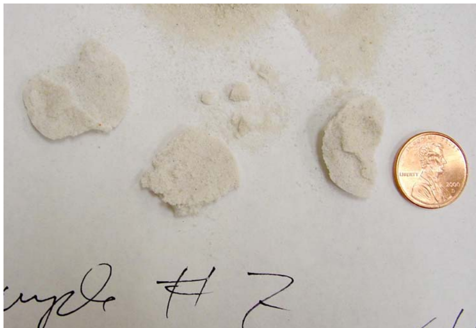
Figure 3.5 Bulk sample following in situ precipitation of LDH in sand pack (Arizona magic sand), followed by drying at 60 °C after removal from the column. Compared to the experiments with mesoporous silicate precipitation (see Figure 4.4), the indurated regions of the LDH sand packs were smaller and noticeably more friable. Material from the lower region of the column is shown on the left and upper region at the right of the image (sample from experiment AZ-7, Table 4.2).
