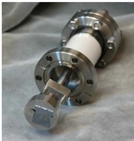
Figure 9. Vacuum assembly used to support and bias the nanotube arrays deposited on silicon-wafer substrates.
