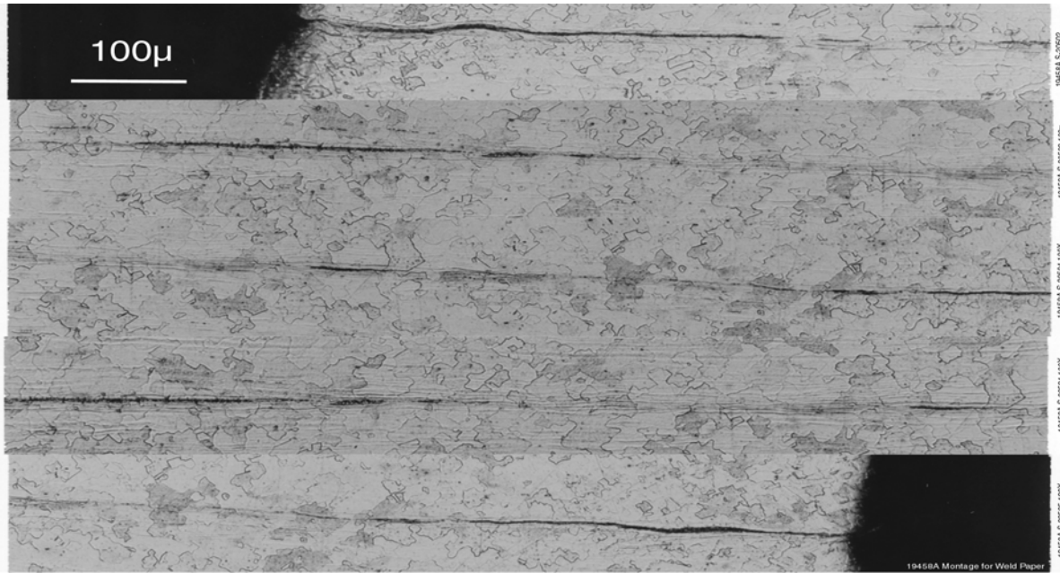
Figure 1. Examples of pinch welds made using contaminated stems.
