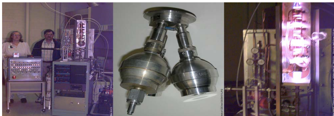
Figure 13. Custom chemical downstream etching (CDE) tool built to clean carbon-contaminated stems. Left: Tool, including control and pumping. Center: fixture to allow three bottles to be cleaned simultaneously. These bottles can be fitted with instrumentation to measure pressures and temperatures during development. Right: Tool with the power on showing the plasma.
