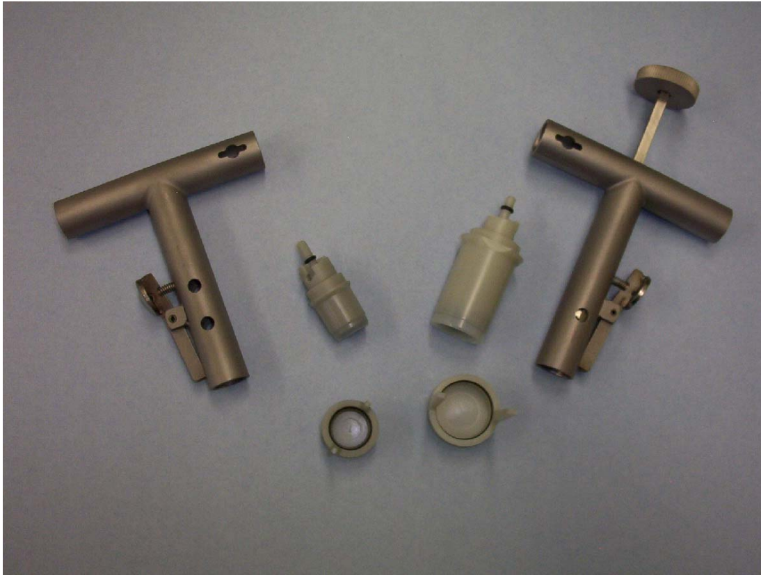
Figure 7. Shown Left to Right, an En Core Sampler T-handle, a 5-Gram En Core Sampler, a 25-Gram En Core Sampler, and an En Core Sampler Extrusion Tool
