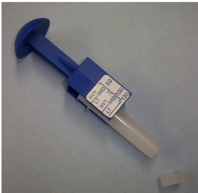
Figure 4b. An Example of a Coring Tool Used to Collect and Transfer a Sample of Soil from the Subsurface Soil Core
