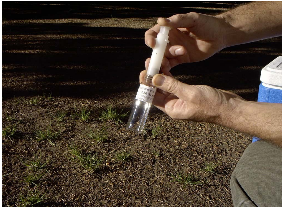
Figure 5. Demonstration of a Soil Sample Being Extruded into an Empty VOA Vial (For actual field work, personnel would be wearing protective gloves.)
