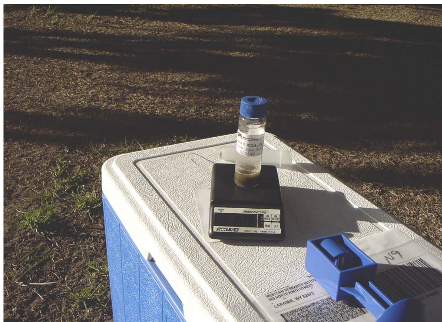
Figure 6. A Soil Sample That Has Been Extruded from a Coring Tool into a 40-mL VOA Vial Containing Methanol
