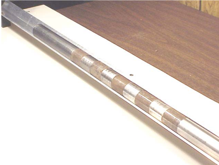
Figure 1. Example of an Accu Core Configuration: Stainless Steel Sampler Sections Arranged in Alternating Order with Clear Acrylic Sections
