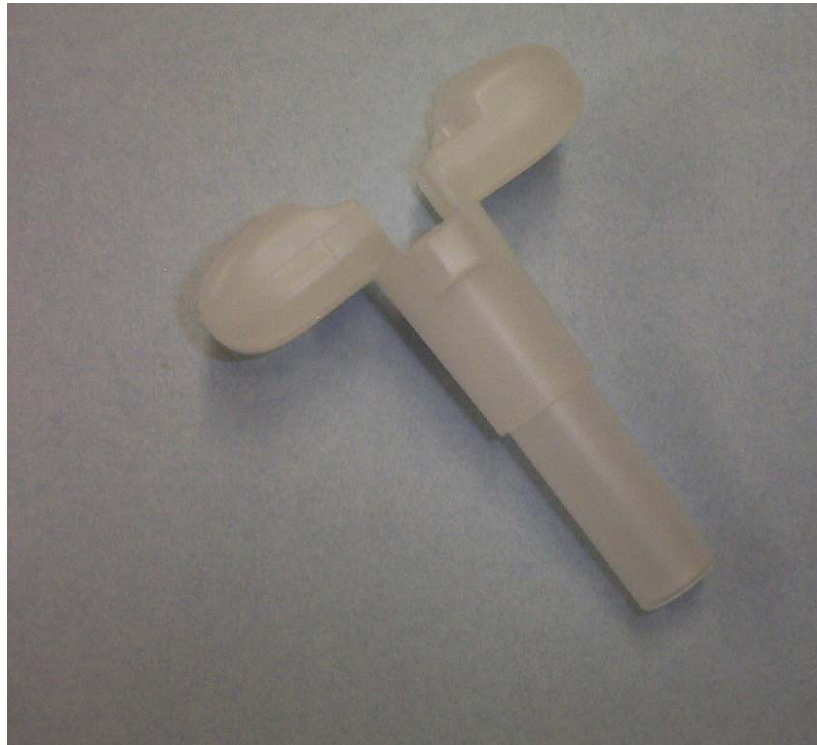
Figure 4c. An Example of a Coring Tool Used to Collect and Transfer a Sample of Soil from the Subsurface Soil Core
