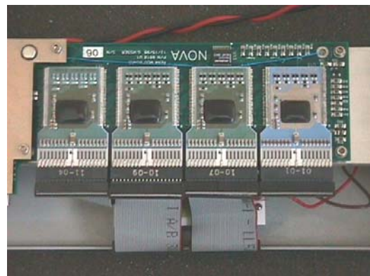
Figure 14. Photograph of 128-channel RENA ASIC system available at RMD for read-out of multi-element CZT/CdTe devices. Each chip has 32 channels & 4 chips are daisy chained. Shaping time is adjustable (0.4 to 6
