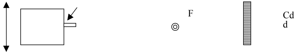
Figure 27. Schematic diagram of the UC-Davis experimental setup used to measure the intrinsic position resolution of the CdTe strip detector ( top view ). The PMT with LSO crystals is shown on the left and moves back and forth as indicated by the arrows. The small 18 F source and the CdTe strip detector (high resolution strips with 0.5 mm pitch oriented vertically) are fixed.
