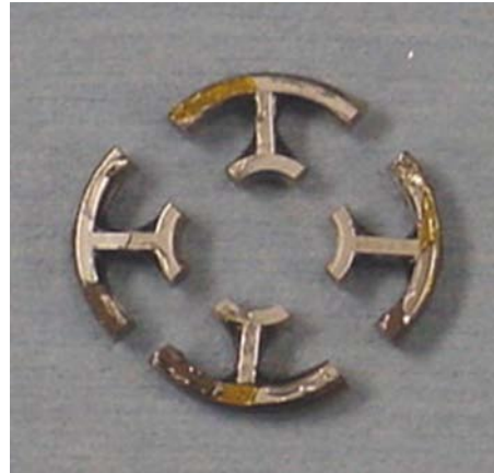
Figure 10: TE stack after quartering to change from parallel to serial electrical connection. This increases the output voltage by 4, and decreases the output current by 4.
