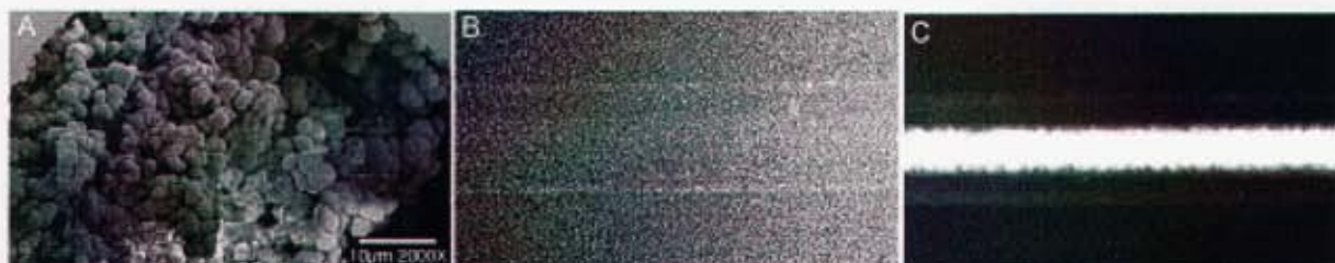
Figure 1.2. Porous polymer monolith are photoinitiated on-chip (A) and bind directly to channel walls. These formed monoliths have no native fluorescence (B), but can be post-functionalized to incorporate any primary amine containing molecule including fluorescent dyes (C), oligonucleotides, proteins, etc.
