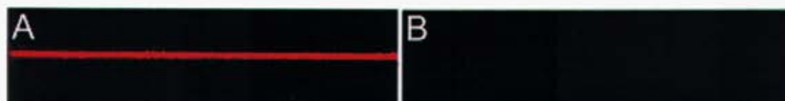
Figure 1.3. Oligonucleotide trapping monolith: These monoliths were functionalized with an Oligo dT. After functionalization the labeled mRNA was dissolved in the binding buffer was introduced to the column, which became bound (A). After a flushing step (not shown) the trapped oligonucleotide was eluted from the column using a salt free TE buffer. This entire process was complete in two minutes.
