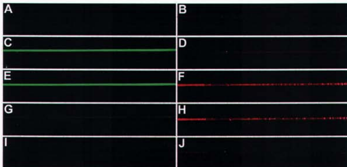
Figure 2.8. Selectivity of PPM preconcentration: Shows the selective adsorption of mRNA (red, right side of figure) over cDNA (green, left side of figure) for preload (A&B), a single volume (C&D), post preconcentration (E&F), washed (G&H) and eluted (I&J). Although DNA is significantly more concentrated than mRNA, only mRNA is left after wash step.
