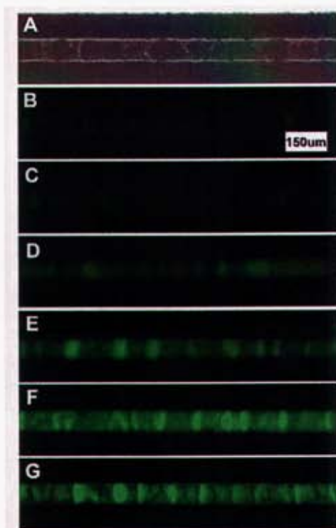
Figure 2.2. Oligo dT binding optimization: Shows a light microscope image of the capillary with monolith (A) together with oligo binding intensity for different times and temperatures. The images are for 60°C for 30 minutes (B) and 60 minutes (C), 90°C for 30 minutes (D) and 60 minutes (E), and 120°C for 30 minutes (F) and 60 minutes (G).
