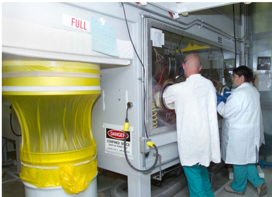
Figure 3-20. Drum packaging system within the Accelerated Retrieval Project.
