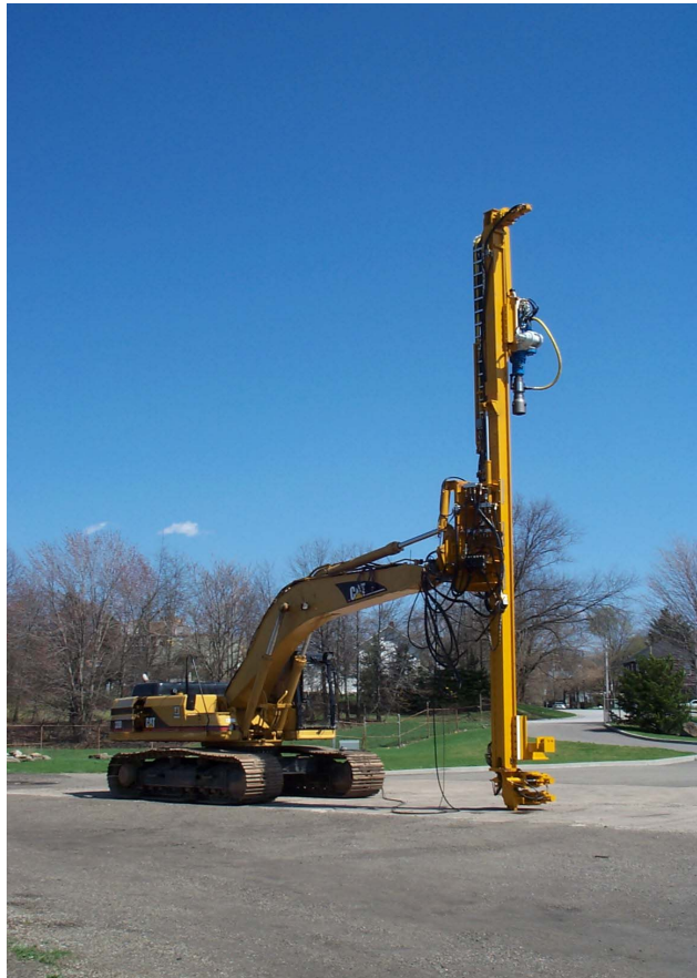
Figure E-30. Trackhoe combined with mast-mounted rotary percussion drill rig.
