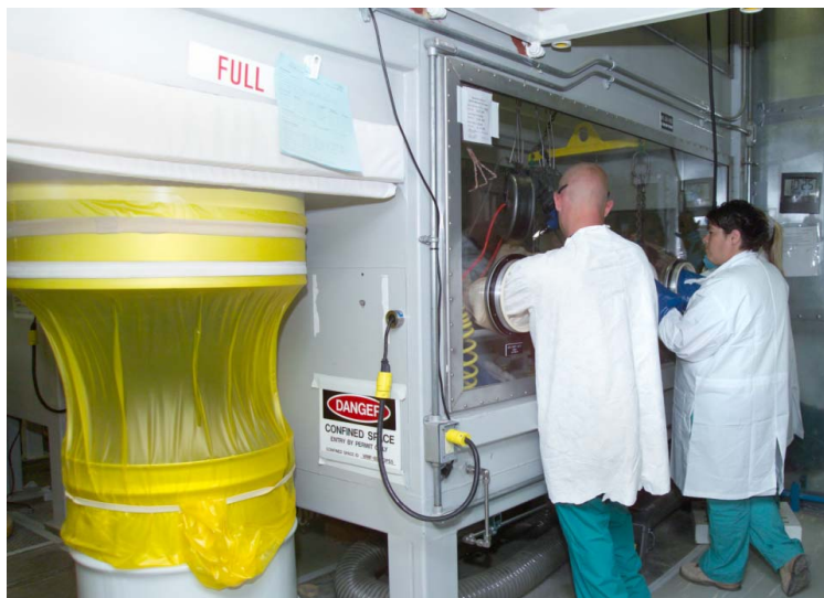
Figure E-5. Drum packaging system within the Accelerated Retrieval Project.
