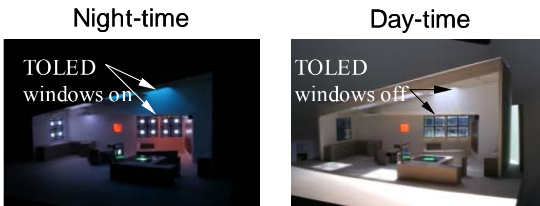
Figure 2. Mock prototype “House of the future” built by UDC containing TOLED sky lighting and windows. Left picture: At night, the skylight and windows turn on and can emit over a range of 'white' colors from warm to cool white. Right picture: During the day, the TOLEDs are off and transparent, so the windows and sky light are transparent.
