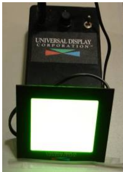
Figure 8. Portable white PHOLED that was coupled to electrochromic device for final deliverable. The device has an area of 25 cm 2 and is only ~1cm thick.
