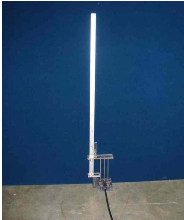
Figure 4.2: Photograph of the device used to measure sand/water and air/water interfaces relative to the top of the probe
