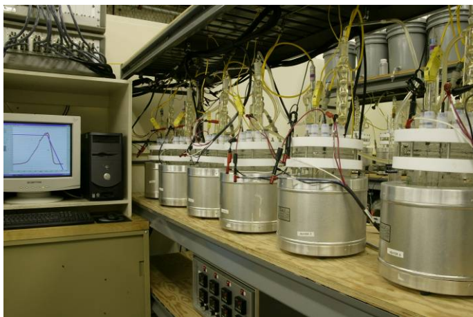
Figure 5. Electrochemical cells used to measure crevice corrosion parameters in different environments.
