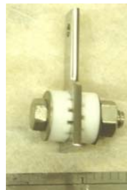
Figure 2. Geometry of specimen used in crevice corrosion tests.
