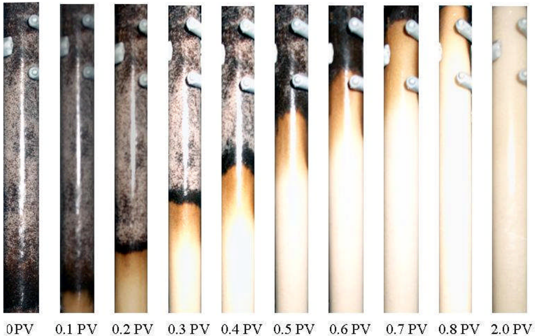
Figure 2.4-8 Photos of silica sand pack at different injecting pore volumes
