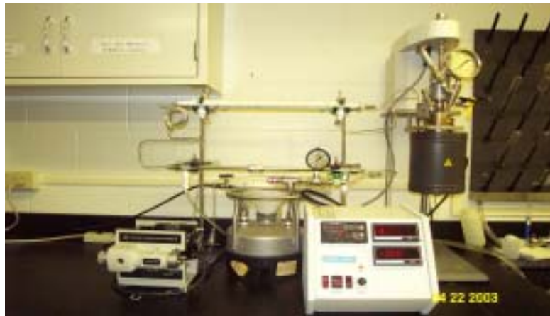
Figure 6-1. Picture of the high-temperature/high-pressure controlled hydrodynamic test system used for the electrochemical experiments. The system is designed to operate at temperatures to 300°C and at pressures in excess of 100b. However, due to the limitations of PTFE (Poly Tetra Fluoro Ethylene) and the need to carry out long term experiments, the maximum operating temperature is currently restricted to 250°C.
