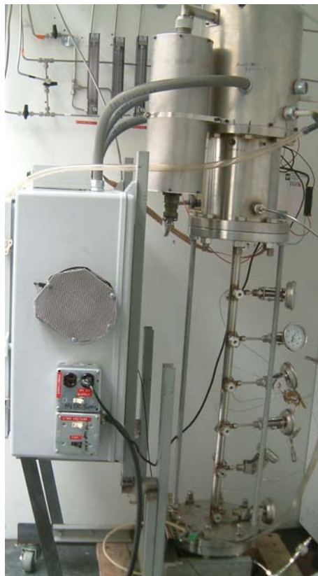
Figure 2. New reactor with viewports and temperature and sampling points.
