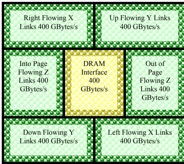
Figure 3: Example Layout of Interconnect Across the Chip
