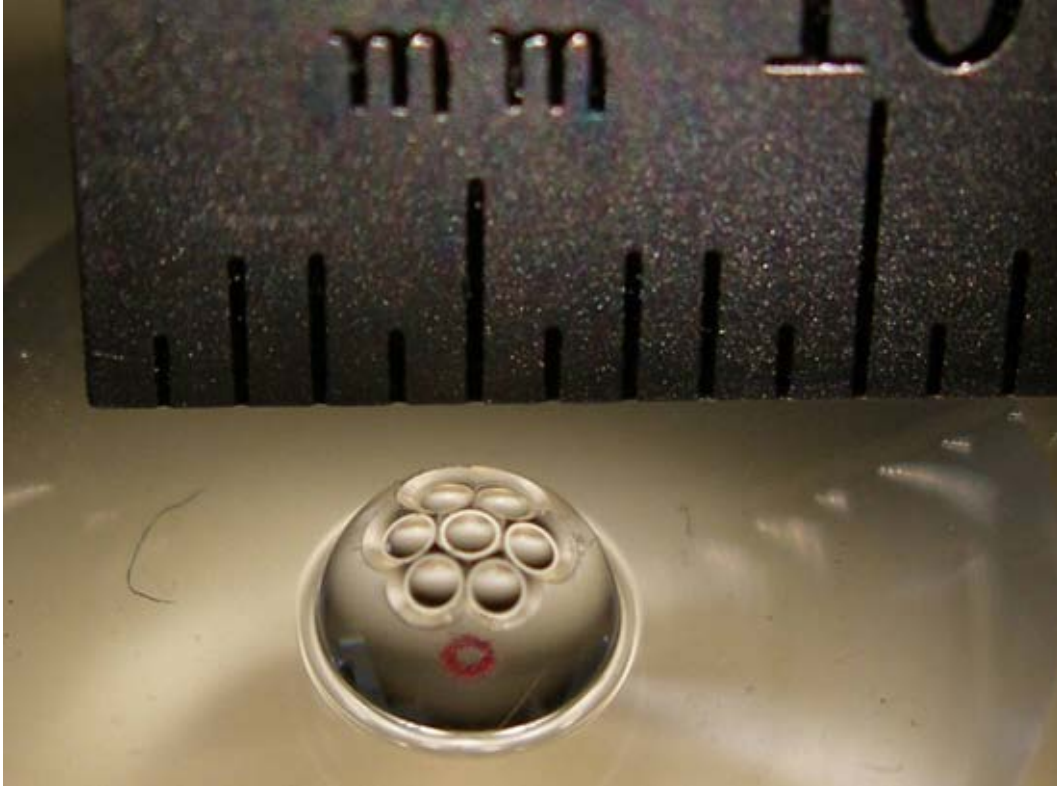
Figure 16. Aspherical Lenslets Milled into the Surface of a Turned Hemispherical Dome
