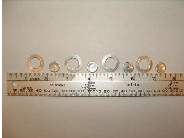
Figure 10: Bluff body structures for Reactor A.
