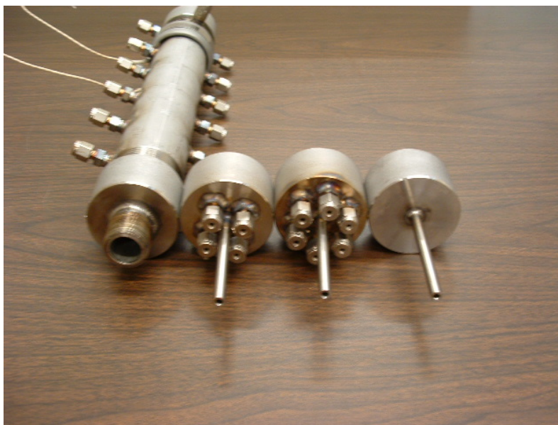
Figure 6: ATR reactor and 4 different end caps (from left to right: acoustic adapter, 4-thermocouple ports, 6-thermocouple ports, regular connection end cap).
