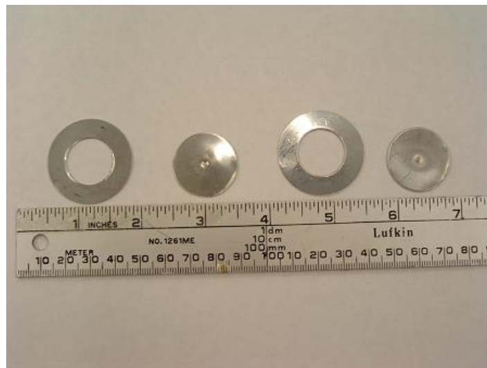
Figure 11: Bluff body structures for Reactor B.
