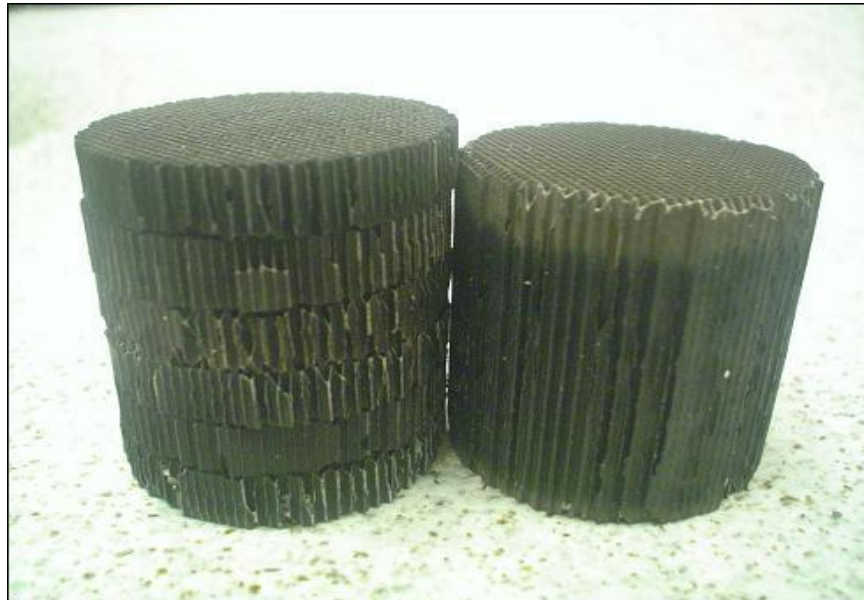
Figure 32: Six, 0.25" catalyst pieces stacked next to a 1.5" catalyst piece.
