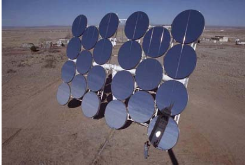
Figure 2-6. The 145-m 2 multi-faceted SM heliostats built by SAIC.
