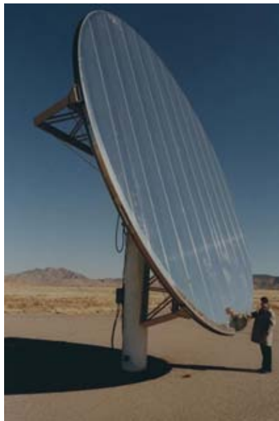
Figure 2-5. Advanced Thermal Systems (ATS) built a 148-m 2 glass/metal heliostat. Science Applications International Corporation (SAIC) and Solar Kinetics, Incorporated (SKI) built four 50 m 2 SM heliostats similar to the one shown.
