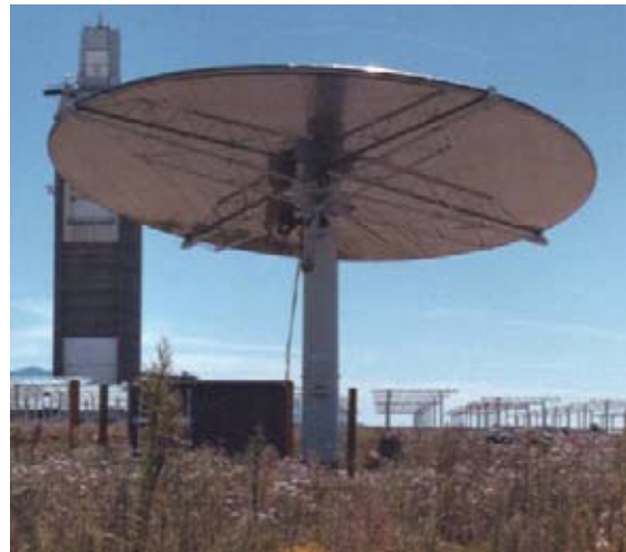
Figure 3-4. SAIC first-generation SM heliostat prototype.
