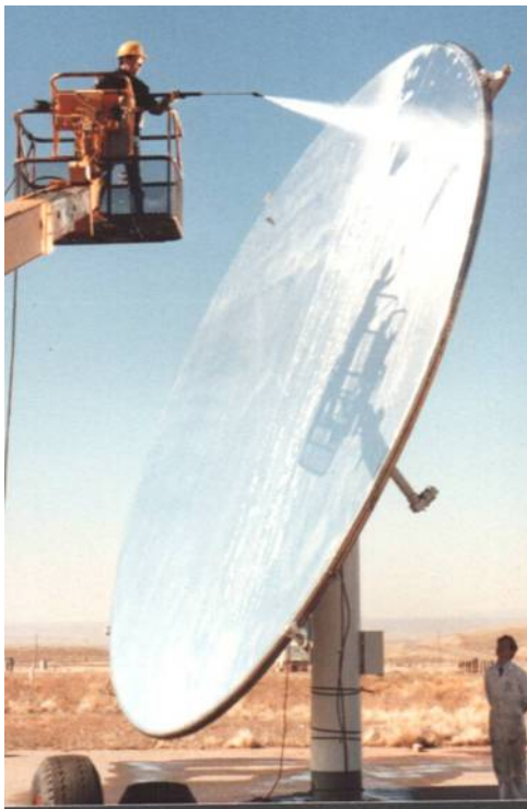
Figure 3-4. SAIC first-generation SM heliostat prototype.
