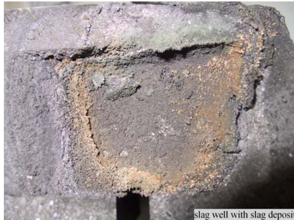
Figure 6. Slag well after 20 hour test with Slag A showing presence of two distinct phases
