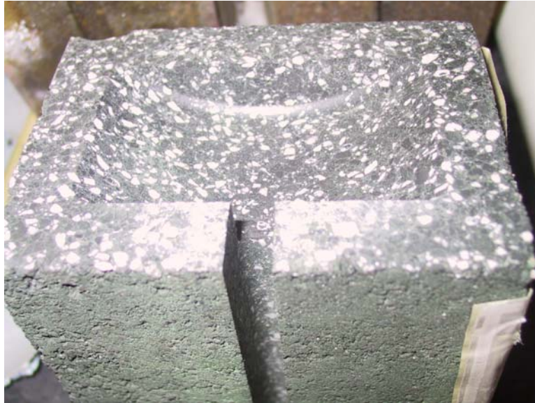
Figure 2. Refractory sample showing slag well and flow channel
