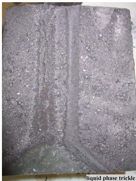
Figure 7. Picture of slag well after 20 hours of testing with Slag A showing little interaction between the slag and refractory.
