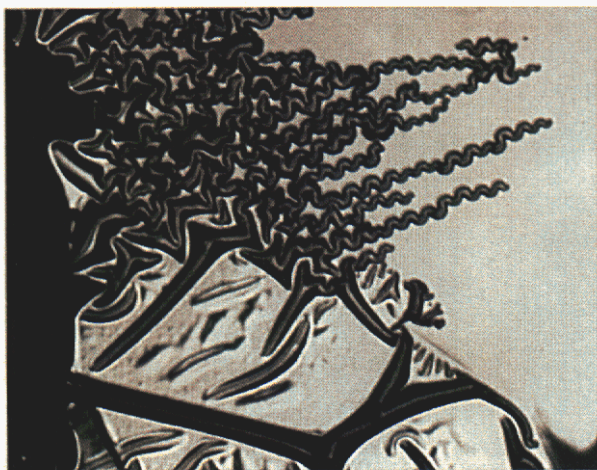
Figure 2.1: Straight and telephone cord buckles formed on the platinum film.
