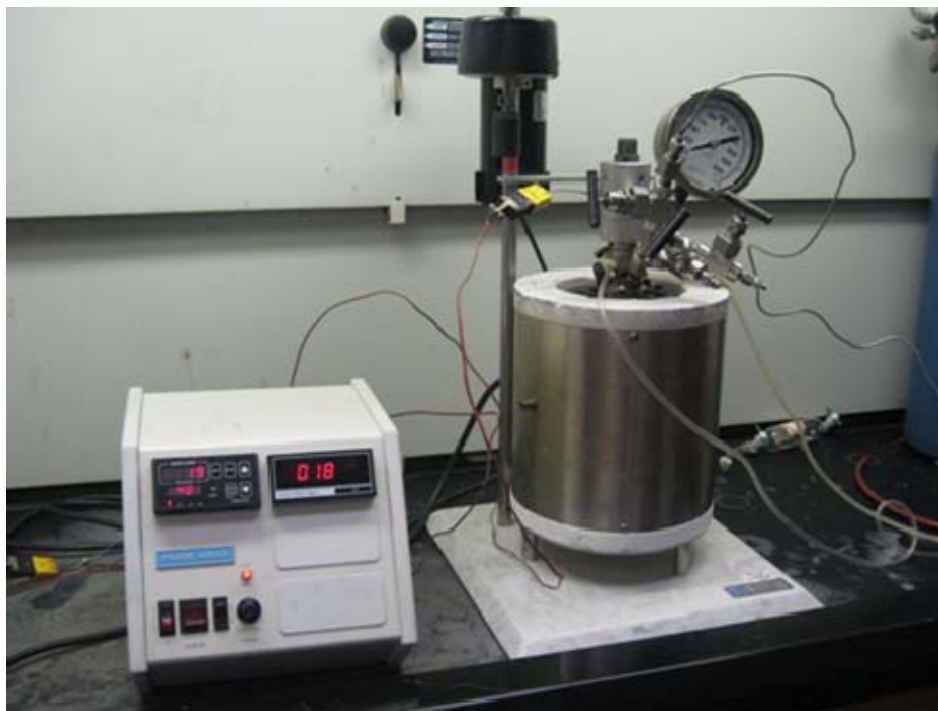
Figure 1. High temperature-high pressure reactor used in heavy oil conversion.
