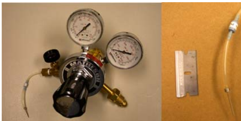
Figure 2. The Regulator/Flow Restrictor Combination Used to Control the Tracer Release and Close-Up of the Restrictor and Filter.
