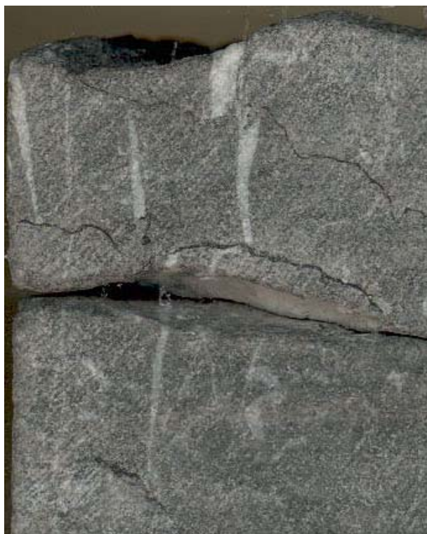
Figure 32. Core from hydrothermally altered Black River in New York showing dolomite-cemented fractures consumed and offset at stylolites. Stylolites postdate dolomitization
