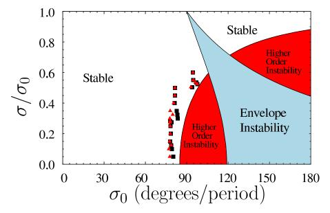
Fig. 5. (color online) Beam stability boundary calculated from a core-particle model for a FODO quadrupole channel. ( $L_p = 0.5 \text{ m}, \eta = 0.5, \varepsilon = 50 \text{ mm-mrad}$ ).
