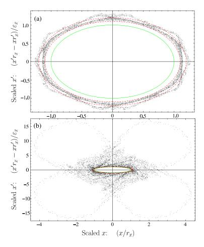
Fig. 4. (color online) Core-particle Poincaré phase-spaces for  $\sigma_0 = 100^\circ$ ,  $\sigma/\sigma_0 = 0.67$  (a), and  $\sigma/\sigma_0 = 0.2$  (b). ( $L_p = 0.5 \text{ m}$ ,  $\eta = 0.5$ ,  $\varepsilon = 50 \text{ mm-mrad}$ ).
