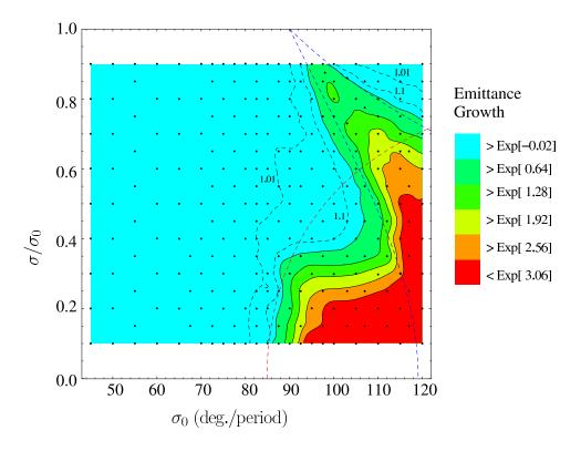
Fig. 3. (color online) Contours of emittance growth for an initial semi-Gaussian distribution in a FODO quadrupole channel. ( $\eta = 0.5$ ,  $L_p = 0.5$  m, and  $\varepsilon = 50$  mm-mrad).
