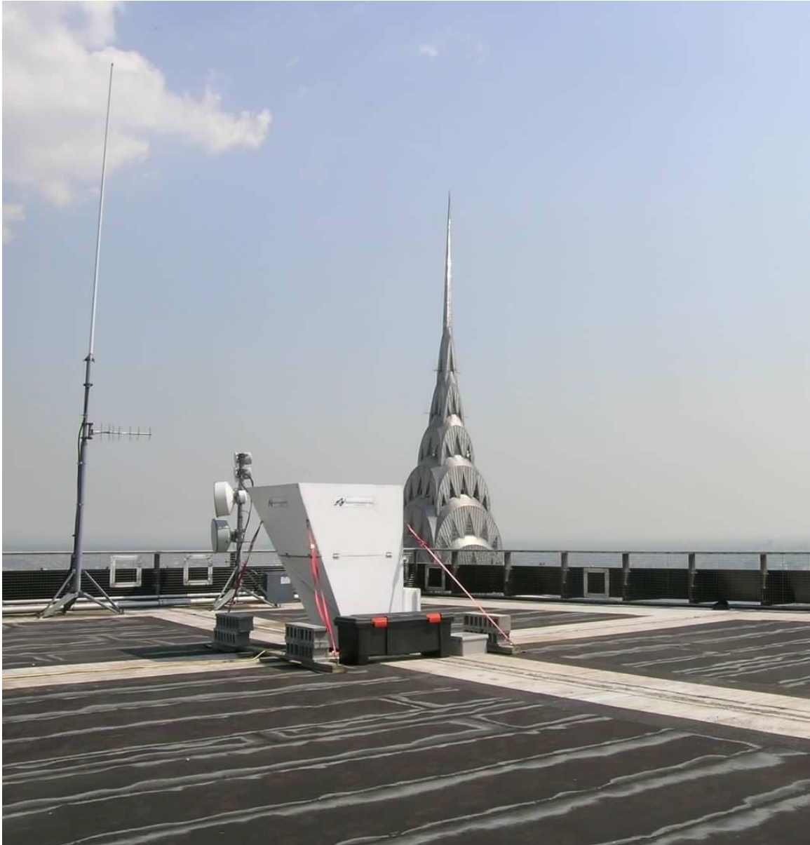
Figure 2 Mini Sodar on the MetLife Building with 3DSonic anemometer in the left background.
