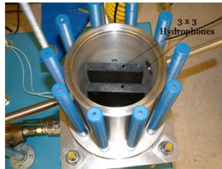
Figure 1: HTHP Re-Circulating System with Acoustic Bubble Spectrometer, 3 in. x 3 in. Hydrophones & Visual Monitoring Equipment
