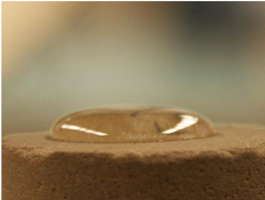
Figure 1. A drop of brine on top of a limestone core aged in crude oil
