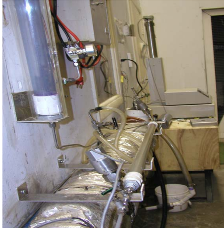
Figure 10. Clear PVC Pressure Transmissibility Apparatus
