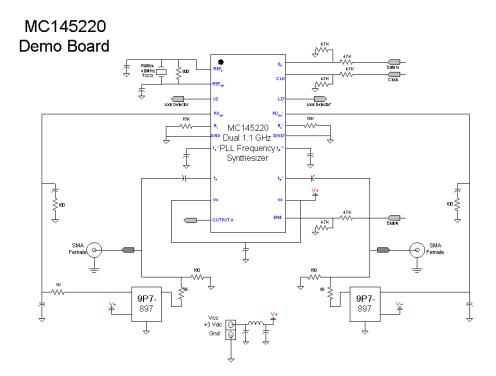
Figure 29 MC135220 Motorola Evaluation Board Schematic Used to measure PLL response
