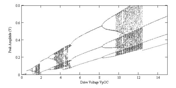
Figure 20 Simulation Bifurcation Plot (Scaled  $t_{rr}$ ) The figure shows the scaled simulation result that is similar to measured results found in Figures 17 and 18.
