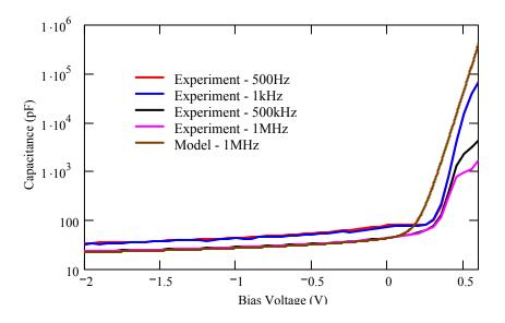
Figure 15 Diode 11 Capacitance
