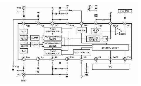
Figure 31 Block Diagram of the Toshiba TB31202FN IC the PLL chip Used in the Radio Shack FRS Radio
