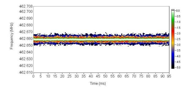
Figure 41 PLL Frequency Response Without RF
