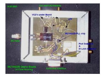
Figure 28 MC145220 Motorola Evaluation Board used to measure PLL response
