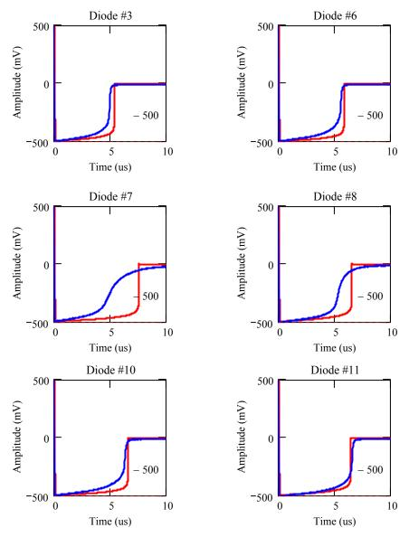
Figure 13 Reverse Recovery Waveforms.
