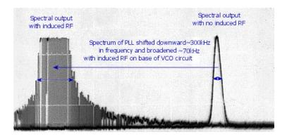
Figure 32 Spectral Shifting and Broadening
