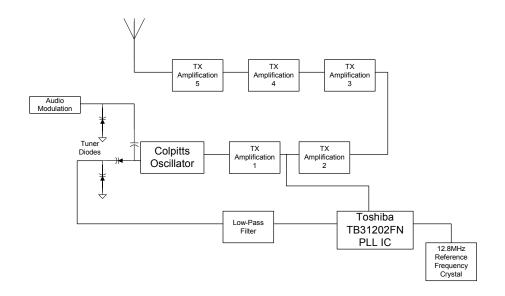
Figure 30 Block Diagram of the Radio Shack FRS Radio RF Section Used to measure PLL response
