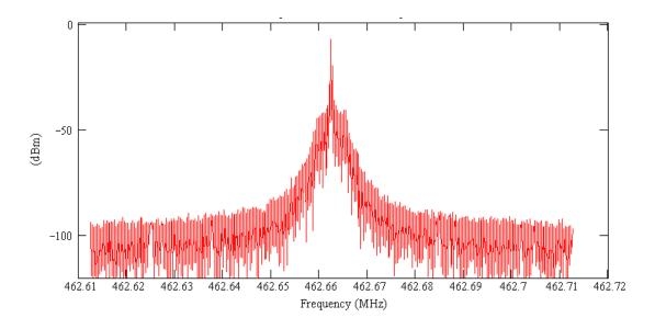
Figure 38 Spectral of PLL without 94 GHz Source
