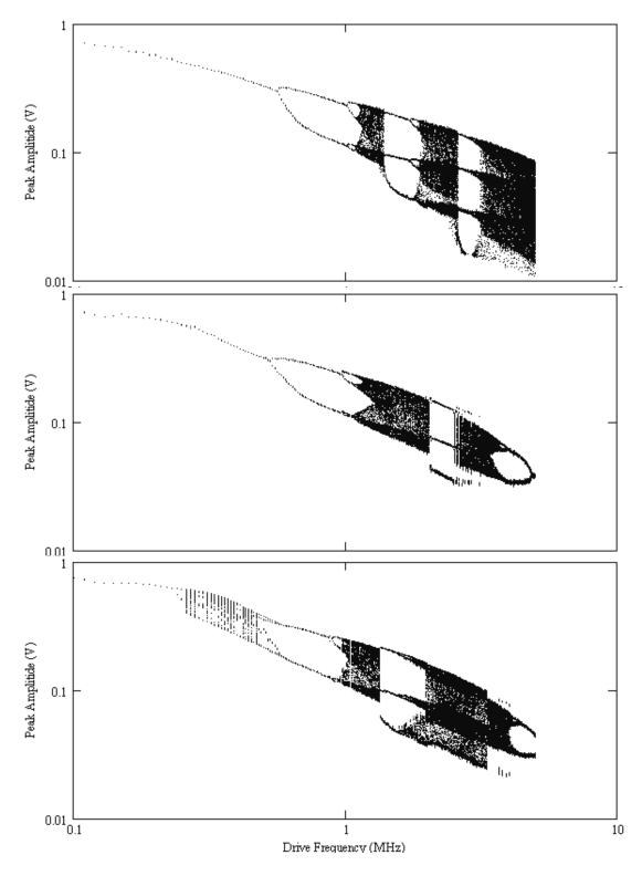
Figure 22 Diodes 8, 10, and 11 Frequency Bifurcation Plots In these plots, the drive voltage is held constant and the drive frequency is varied. As with the voltage bifurcations plots, the response transitions between period and chaotic behavior.
