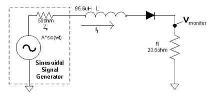
Figure 16 Diode Resonator Circuit commonly referred to as the Linsay Circuit
