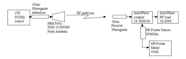
Figure 36 Power Measurement Layout
