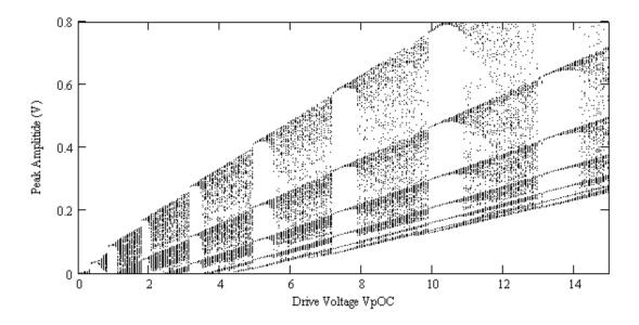
Figure 19 Simulation Bifurcation Plot (Un-scaled t<sub>rr</sub>) This figure shows un-scaled simulation results. These results differ significantly from measured results shown in Figures 17 and 18.
