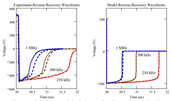
Figure 14 Experiment and simulation results of one versus eight pulses. The solid lines show the recovery response of a single pulse and the dotted lines show the response of the last pulse in a pulse train. The greater drive frequency shows a larger difference between experimental results and measured results.
