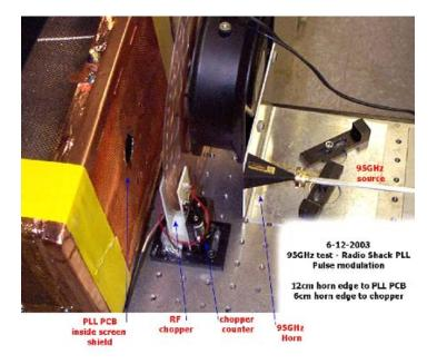
Figure 37 Setup of 95GHz Test at 12cm
