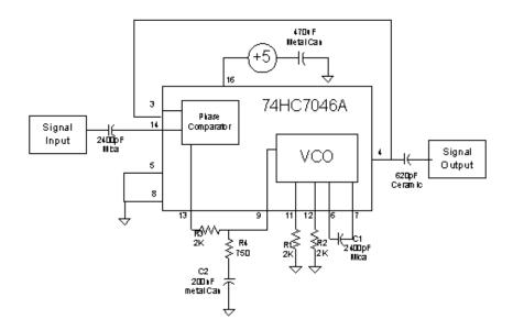
Figure 26 74HC7046A PLL Circuit
