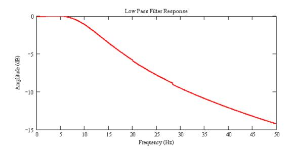
Figure 46 PLL Low Pass Filter Response
