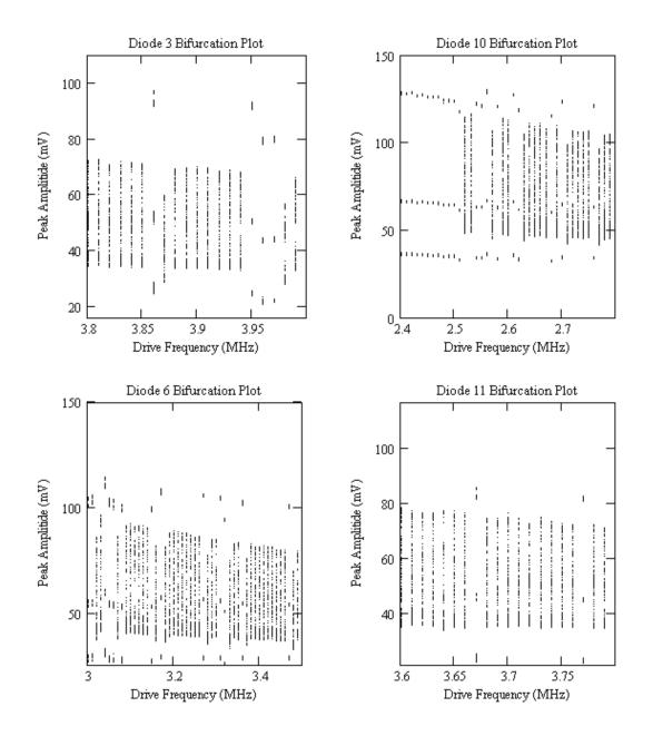
Figure 23 Frequency Bifurcation Details for Diodes 3, 6, 10, and 11. This figure shows a blowup of Figures 21 and 22. On this frequency scale, one can see how readily the circuit response can change from periodic to chaotic.
