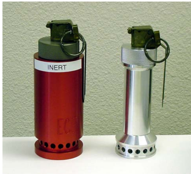
Figure 1: Redesigned flashbang device. Prototype design is on the left, while the redesigned body is on the right. While the redesigned body is smaller in diameter and shorter in length, the internal volume and dimensions are preserved.
