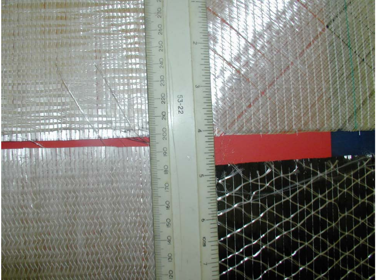
Figure 1.1: Constitutive fiber complexes. (Clockwise from upper right: 12 oz/yd^2 double bias glass, 15 oz/yd^2 unidirectional carbon, 6 oz/yd^2 unidirectional glass, 16 oz/yd^2 unidirectional glass.)
