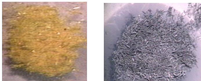
Figure 3. Left: Pristine needles of \text{Mo}_6\text{Cl}_{12} , Right: Gray needles formed by ageing at 300^\circ\text{C} for one hour.
