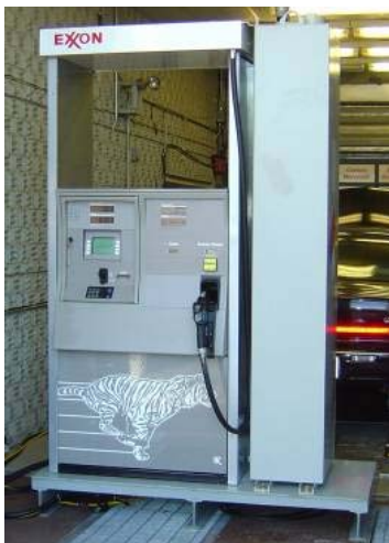
Figure 53. Prototype co-fueling dispenser.
