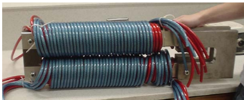
Figure 11. Photograph of Electromagnet after Modifications
