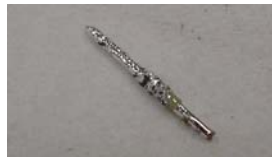
Tungsten did not experience significant change in dimensions
