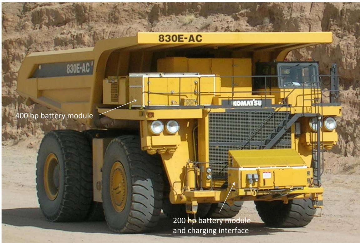
Figure 1 – 240-ton hybrid OHV in test at Komatsu Proving Grounds
