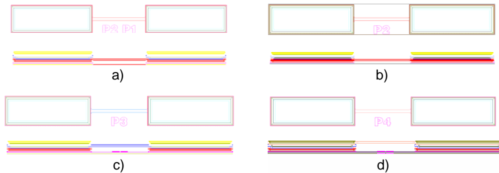
Figure 4: Top and side views of thermal conductivity test structures: a) P1P2A b) P2A c) P3A and d) P4A. The side view of a test structure with an underlying via is identical to those shown above except the substrate directly under the beam is removed. The vertical scale of the side view is enlarged to improve visibility.
