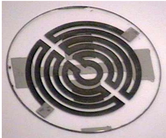
Figure 8. Integrated back-side emitter wafer heater.
