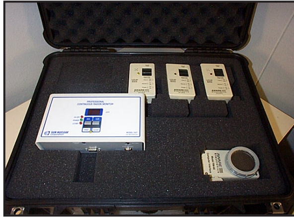
Figure 2. Top layer of sensor unit displaying the 1027 CRM radon monitor (large box), three LCD-60 displays for PMI-30 and RM-80 sensors (L to R:) gamma, neutron, beta, and the RM-80 interface sensor (lower right)
