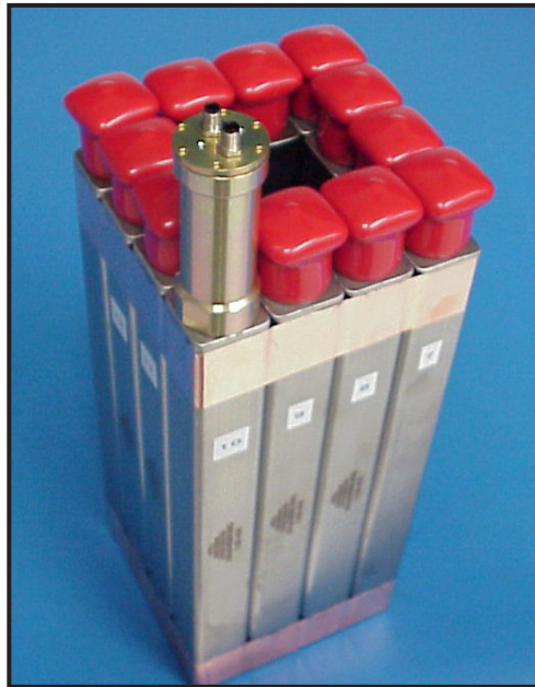
Figure 1. Array of 12 detectors with electronics module attached to one
