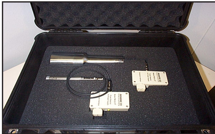
Figure 1. Bottom layer of one sensor unit displaying two PMI-30 interfaces to NaI and neutron sensors containing ^3\text{He}
