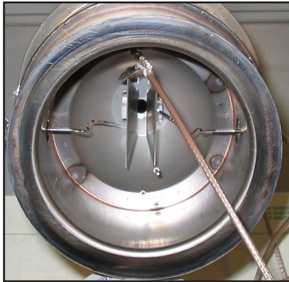
Figure 2. Phosphor end view of deflection section
