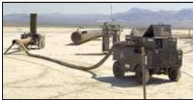
Figure 1. C-130 start cart and existing NPTEC mini-stack
