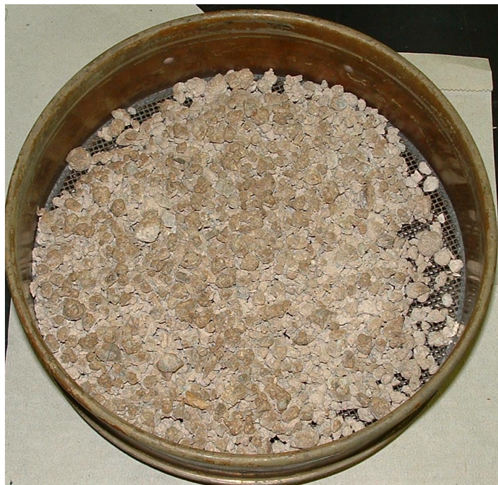
Figure 8: Agglomerated ore after air-drying for 24 hours, before soak test in simulated raffinate. These agglomerates were made using only raffinate as binder.
