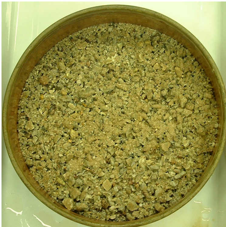
Figure 12: Raffinate-bonded agglomerates removed from simulated raffinate after 20 minute immersion. The agglomerates have almost completely broken down.
