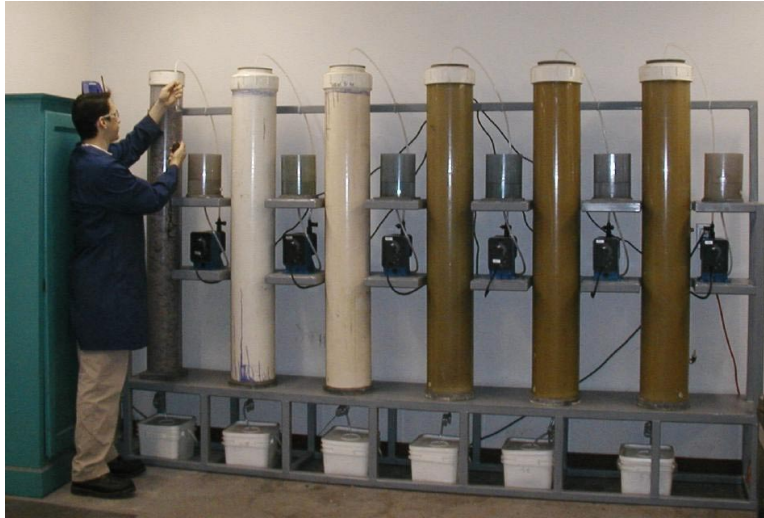
Figure 4: Leaching columns provided by Phelps Dodge set up for leach testing at Michigan Technological University. These columns are used for long-term testing for periods of several months, and provide the closest simulation of actual industrial heap-leaching behavior that can be achieved in the laboratory.
