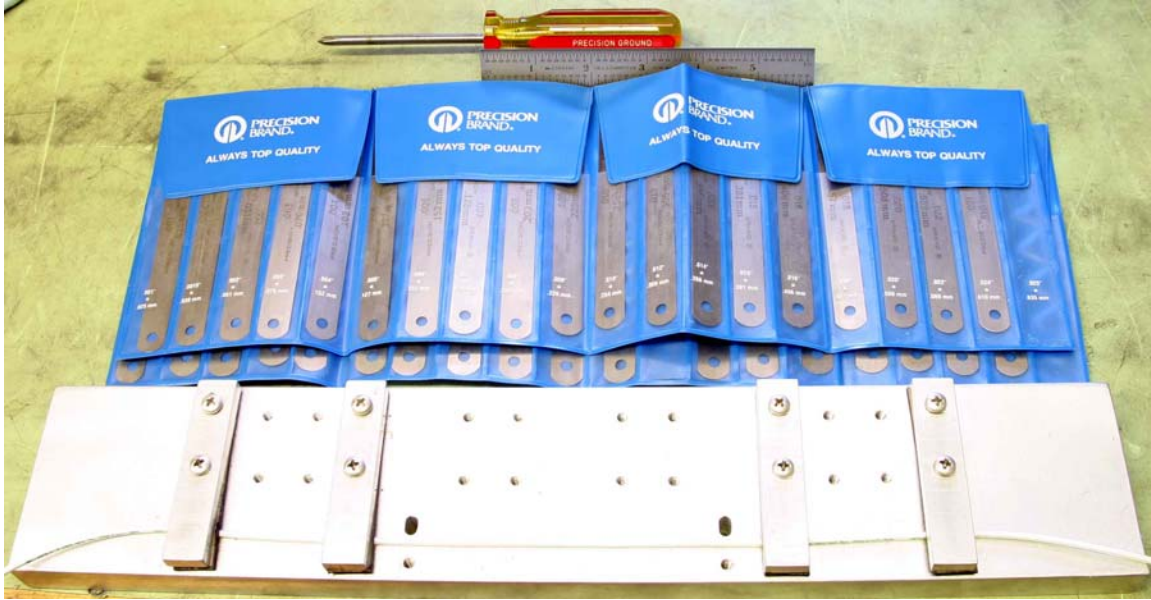
Figure DT2-4. Breach Defect Cutting Fixture and Feeler-Gauges
