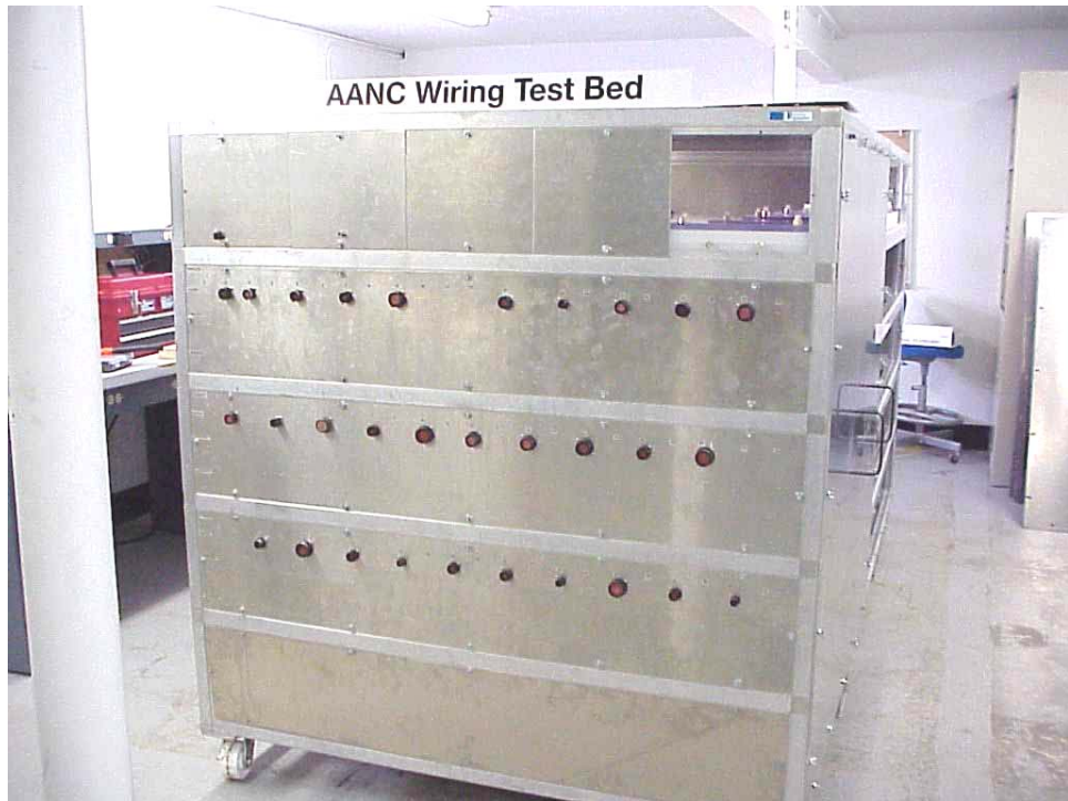
Figure 4. Assembled Wire Harness Enclosure
