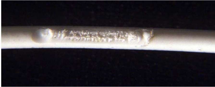
Figure DT1-4. Partial Wire Insulation Abrasion
