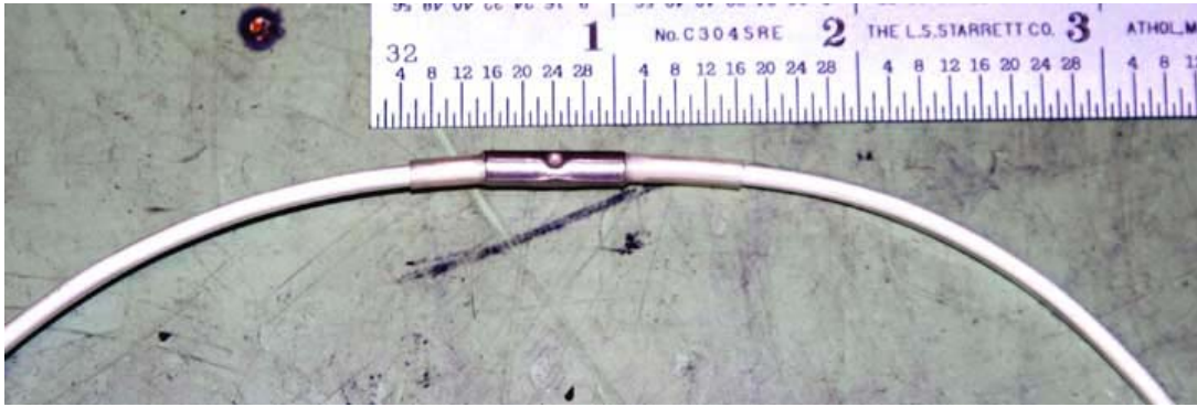
DT7-1. Example of Type I Un-Crimped but Heated Faulted Splice
