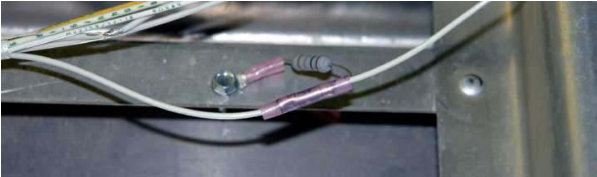
DT10-2. Resistor Used to Simulate a Partial Short
