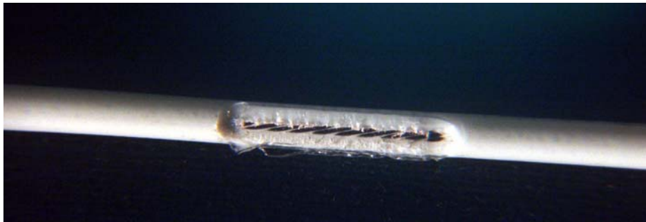
Figure DT1-5. Full Wire Insulation Abrasion Exposing Conductor
