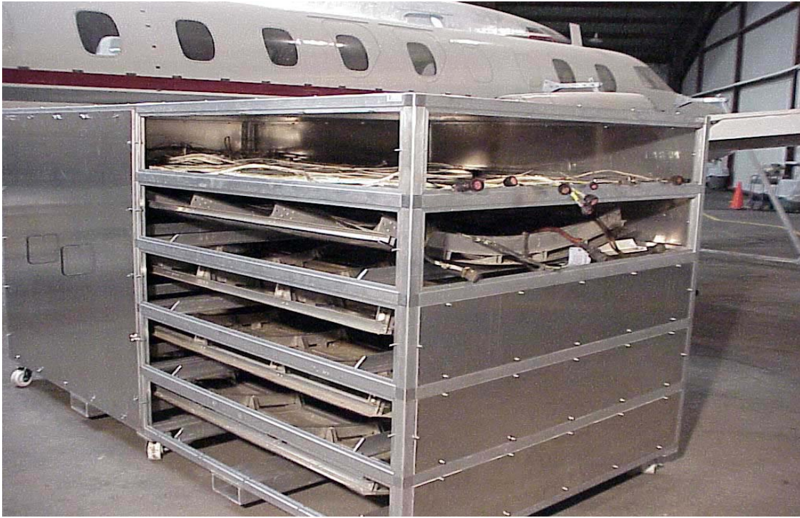
Figure 2. Partially Assembled Wire Harness Enclosure
