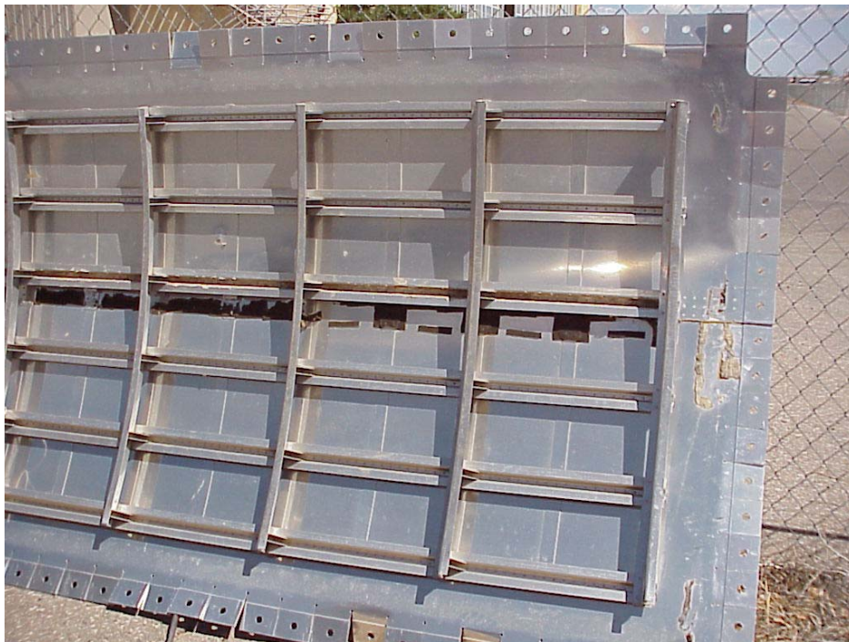
Figure 3. Boeing 727/737 Type Ribbed-Structure Segment Fabricated by Foster-Miller
