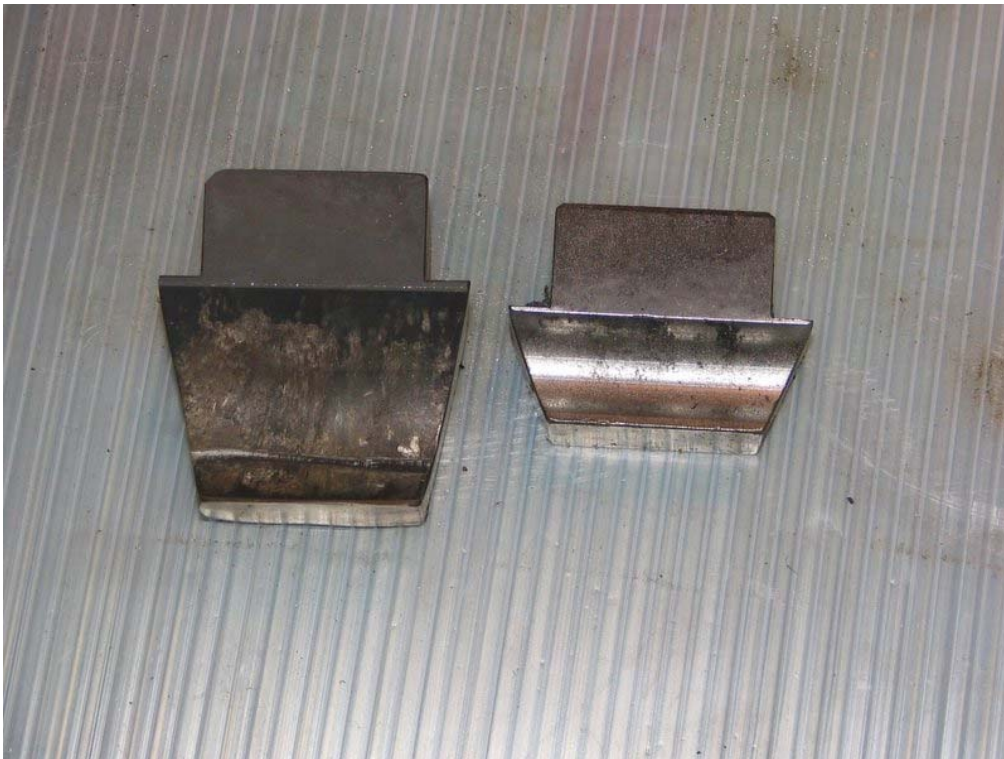
This shows the new tooth design, on the left, and the old design on the right. The new design has a much larger “bite” and can grab more of the carpet and pull it into the system. The rotor is smaller and has fewer teeth.
