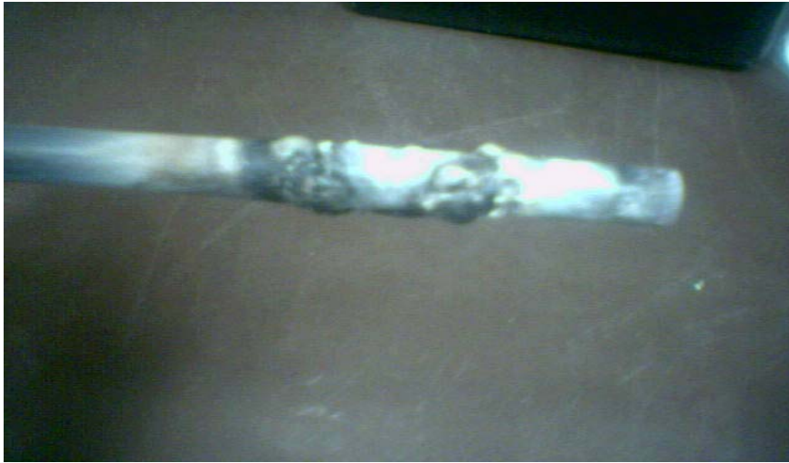
Figure 5-86 Photograph of the failed test heater for the 5000 ppm lithium metaborate particulate deposition test (68.9 bar).
